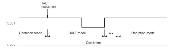
When the RESET signal is applied to release the HALT mode, the RESET input makes a transition from low to high, then an operation mode is entered.
