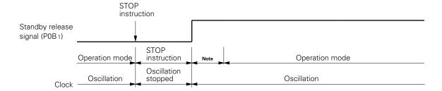
**Note** The HALT mode remains effective in this period, waiting for the generation of clock pulses to settle. At least eight clock pulses on the OSC<sub>1</sub> pin cause operation to start.
