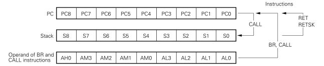
In Fig. 2-1, AHn, AMn, and ALn ( $0 \le n \le 3$ ) indicate bit positions in a 16-bit instruction as follows:
